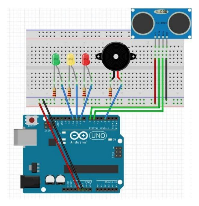
**Buzzer** : pin 3 **Ultrasonic Sensor**: Echo = pin 6 Trig = pin 7
